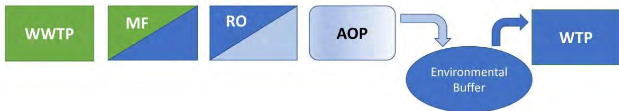
Figure 3-1 Demonstration Project Process Flow Graphic
