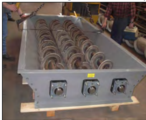
Figure 11 Internal Screws in surge bin live bottom hopper
