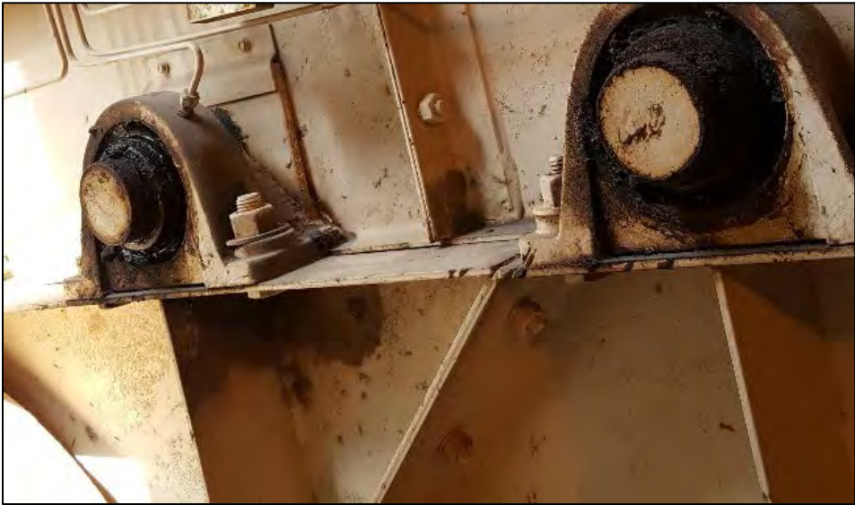
Figure 8 Interior Corrosion in Bulk Amendment Bin
