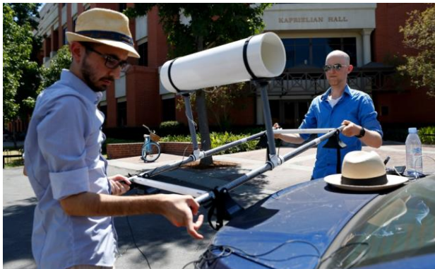
GEORGE BAN-WEISS, right, and Arash Mohegh remove a mobile thermometer from a car. (Gary Coronado Los Angeles Times)
