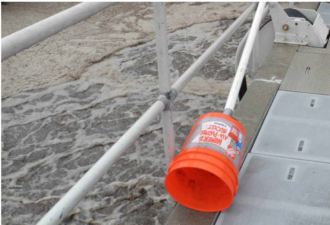
Picture 4 (top) showing off-gas analyzer, author and bucket hood on 1.5 in, diameter PVC pipe. Picture 5 (bottom) showing a close up of the bucket hood.
