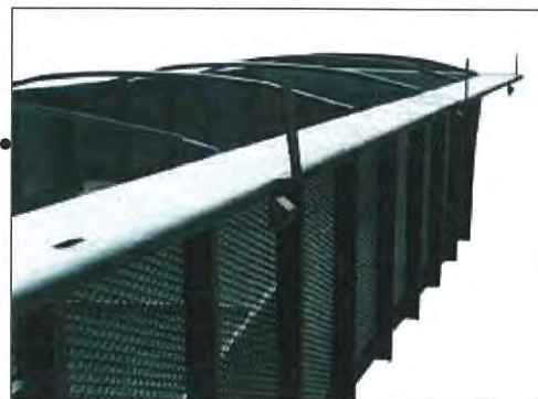
Removeable dewatering shells and disposable liners make clean up easy.
