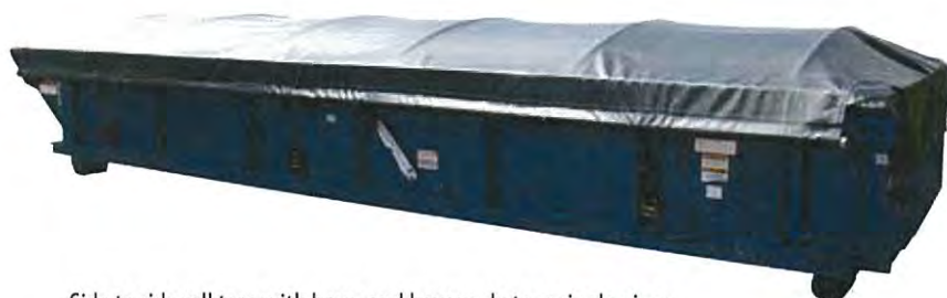
Side to side roll tarp with bows and bow pockets or single piece, side-to-side plastic or aluminum lids.
