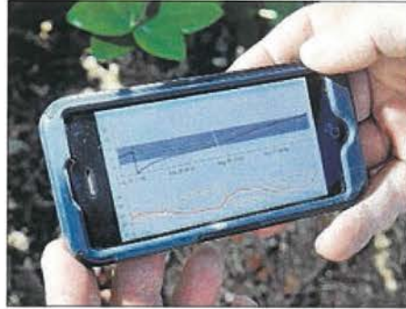
Will Gerry, owner Coastal California Blueberry, uses the Hortau irrigation management system, which measures the amount of water moisture and content of the soil.
