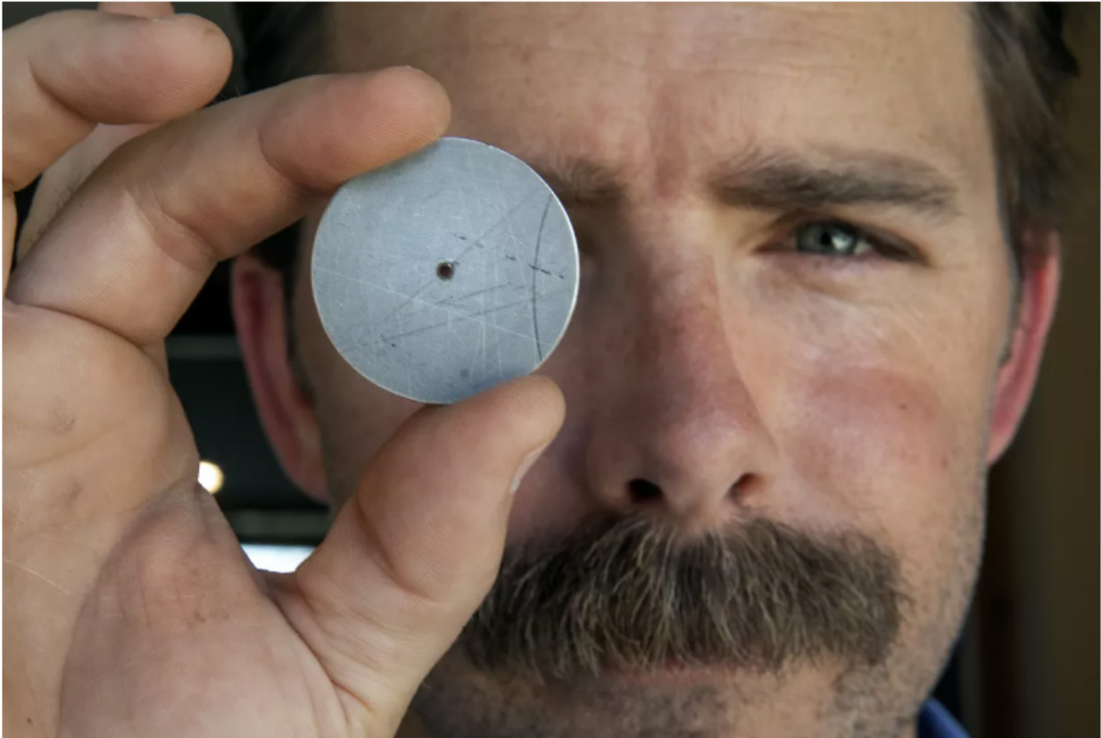
Cason Gilmer, a senior field customer service representative for the Las Virgenes Municipal Water District, holds a water flow restrictor device he designed. It will be used to reduce water flow to customers who repeatedly exceed water usage. (Mel Melcon / Los Angeles Times)
