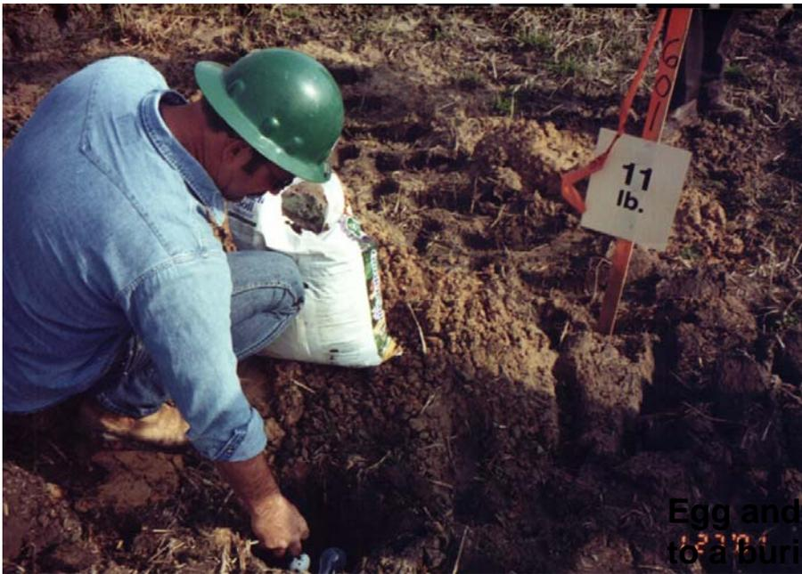
**In a Controlled Test, Buried Raw Eggs and Light bulbs Survive Vibration 10 times greater than that allowed for this work (5.0 versus 0.5 in/s)**
