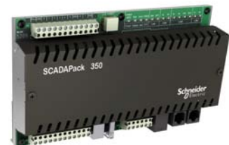
Figure 3-1 Schneider Electric and Allen Bradley Ethernet PLCs
