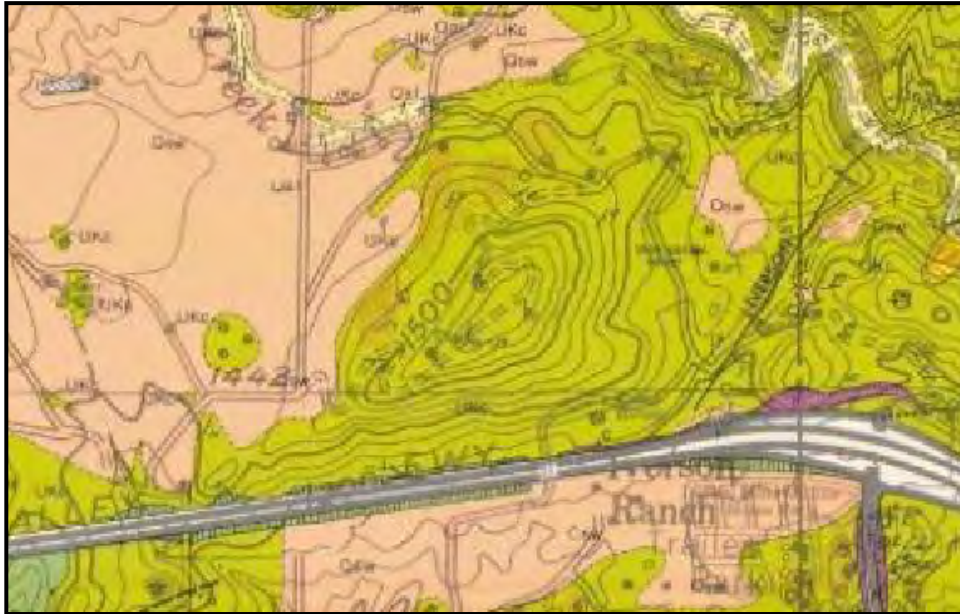
Figure 8: The 1981 Oat Mountain USGS Map, showing the project development footprint (center), which is entirely within the Chatsworth Formation (green).
