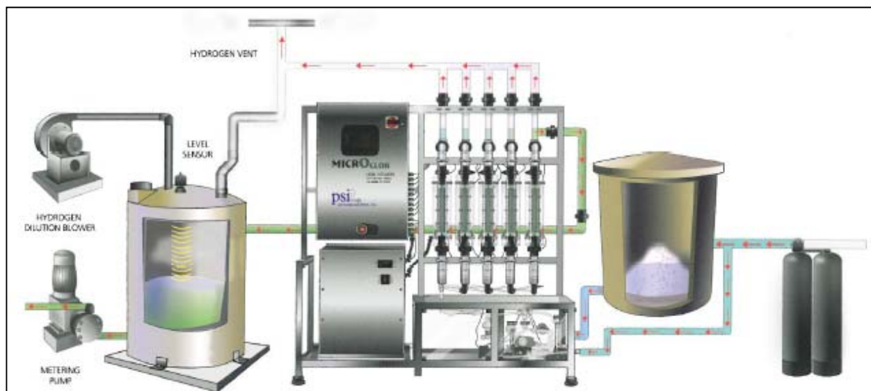
Figure 7 On-Site Sodium Hypochlorite Generation System
