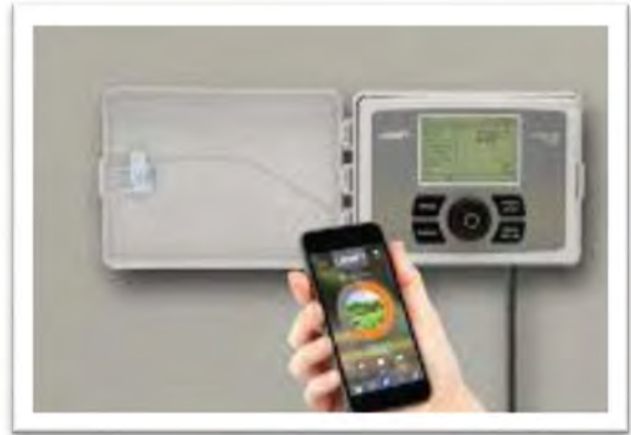
Figure 1 - WBICs can be programmed and monitored with a Smart Phone
